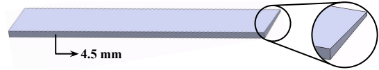
Fig. 10. Triangle-shaped 3D printed structure attached to both walls of the fog outlet to reduce the fog outlet width to one-fourth, 3cm from 12cm. A 3-mm version was also created to reduce the fog outlet width to half.
