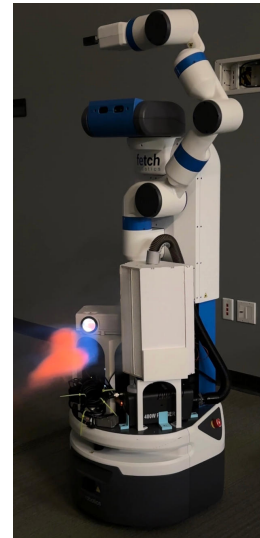
Fig. 1. The fog screen-robot system. A human icon is projected, which is useful in search-and-rescue scenes to indicate the sign of life of a human victim. A video is available at https://osf.io/pxsfy . To be discussed in Section VI, we also simulated a construction site scenario.
